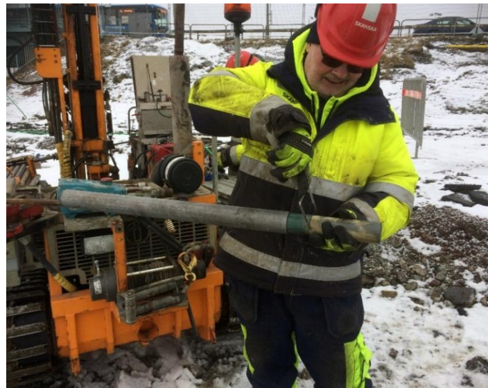
Figure 4.6: Separation of the tubes after sample collection.
