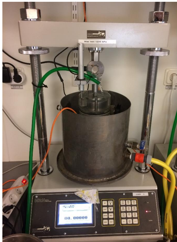
Figure 4.8: One of the CRS in the laboratory at Skanska.
