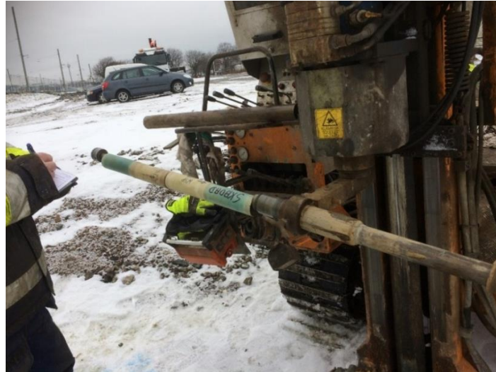
Figure 4.5: Preparation of the tubes on the piston sampler.
