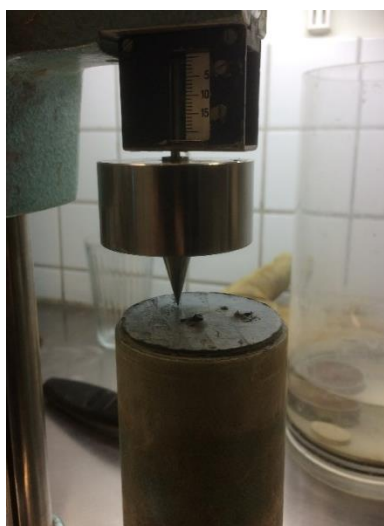
Figure 4.7: Examination of undisturbed shear strength using the fall cone test.
