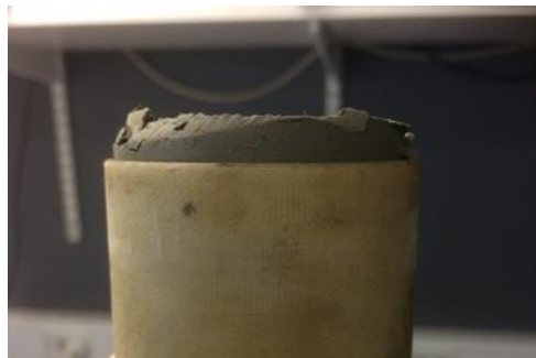
Figure 5.8 Swelling of the sample collected from 25 m, 8 days after sampling. Similar on the other end.
