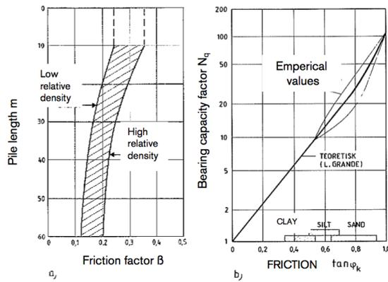
Figure 1: Values of the friction factor  $\beta$  and the bearing capacity factor  $N_q$  (From “Norsk peleviledning”)
