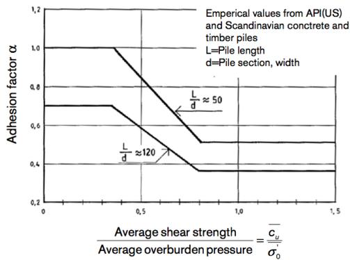
Figure 2: Values of the adhesion factor  $\alpha$  (From "Norsk peleveiledning")
